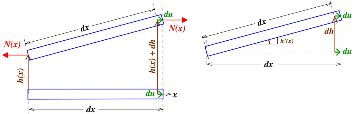
Figure 2. Axial end displacements due to transverse displacements, without axial deformation.
