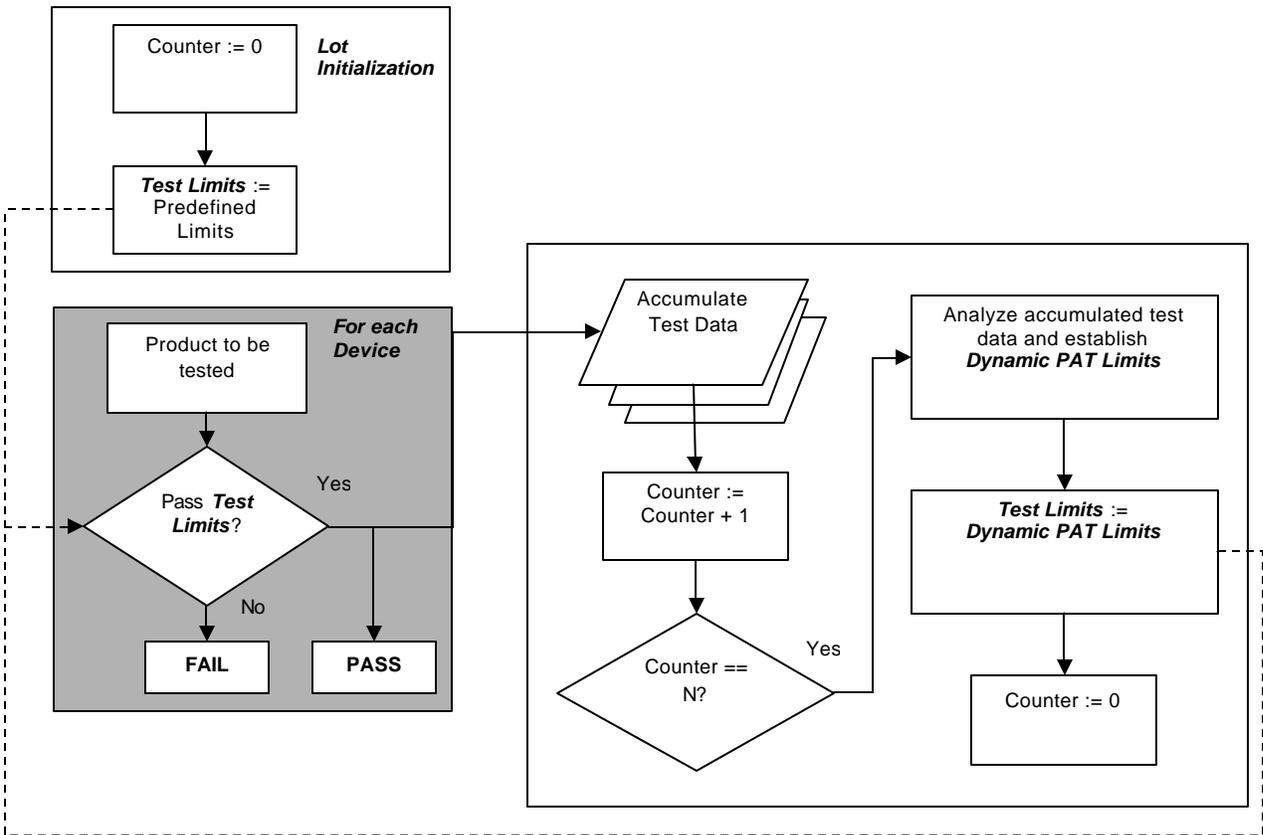
Figure 3: Dynamic PAT Application for Packaged Product Tests
