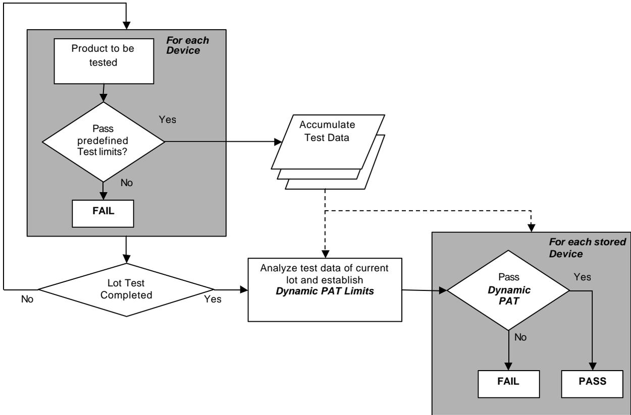
Figure 2: Determining Dynamic PAT Limits (Probe or Serialized)
