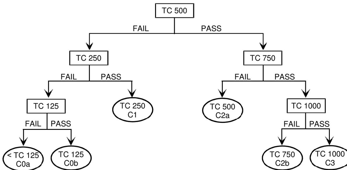
**Figure 1: Recommended Discrete Semiconductor CDM ESD Test Flow Diagram**
