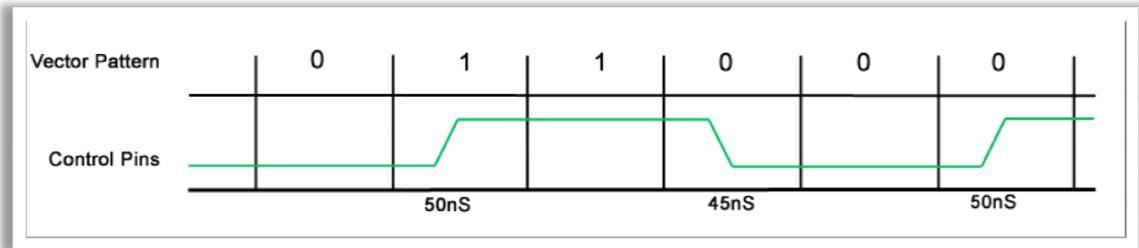
2: Pin group “Data\_pins” will change state within each vector. This is a variation of Surround by Compliment or XOR format and is useful for Address and Data buses to allow set-up and hold timings.
