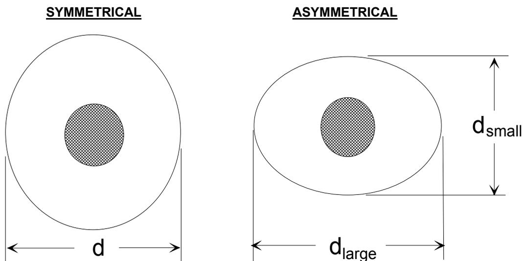
**Figure 2: Ball Bond Diameter Measurement (symmetrical vs. asymmetrical)**
